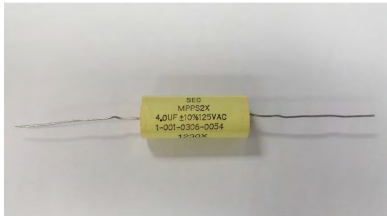
Figure A – Suspect supply of capacitor C306 (AI 2 P/N: 1-001-0306-0054)
